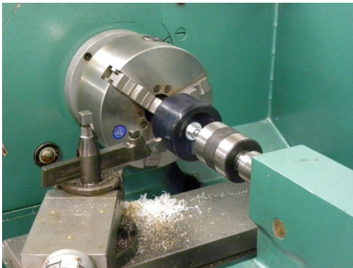
Figure 8: Lathe Groove in Guide Wheel
