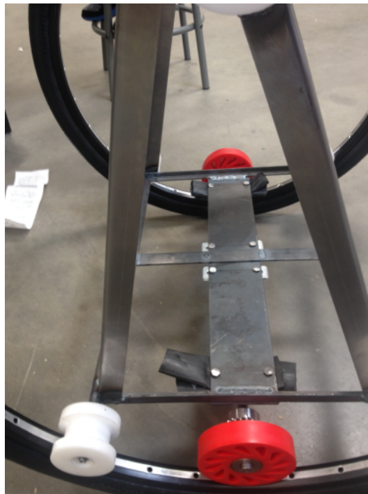
Figure 6.1.6: Drive Train Assembly Drive Wheel on Bike Wheel Rim
