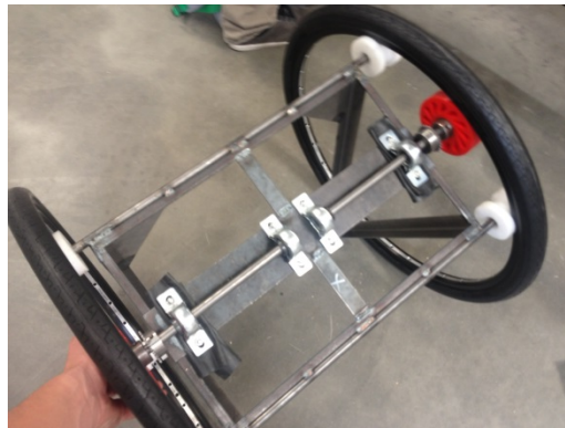
Figure 31: Bearings with Adjustments
