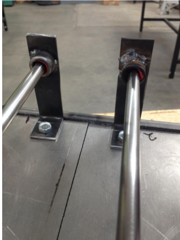
Figure 6.1.4: Modified Linear Leveling Rail Mounts
