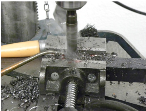
Figure 18: Drilling with 5/8 Bit
