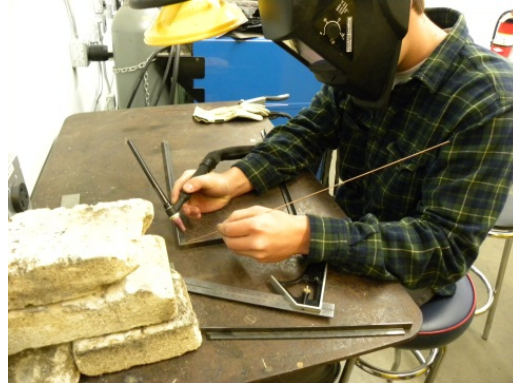
Figure 2: Welding Steel Frame
