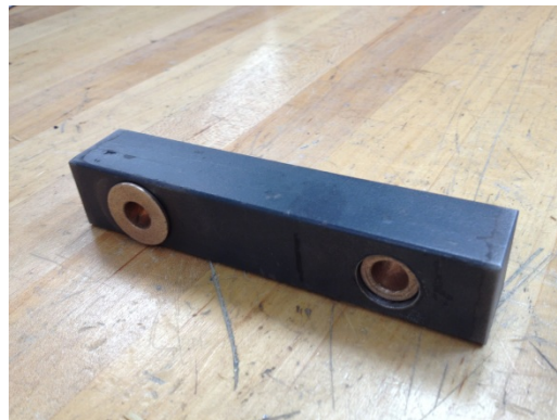
Figure 19: Finished Weight with Bearings
