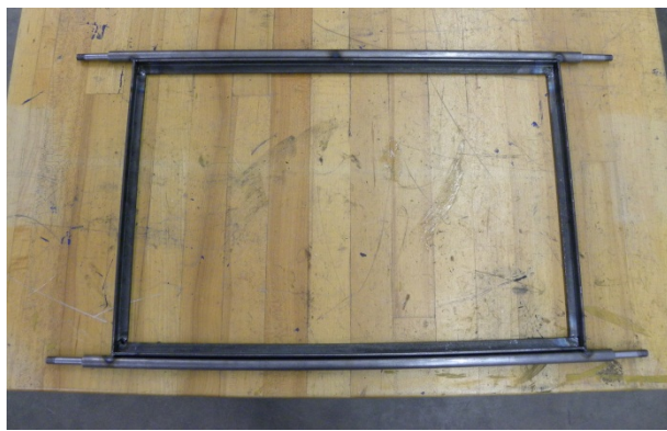
Figure 26: Guide wheels axels welded to frame
