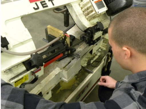
Figure 1: Cutting Angle Iron
