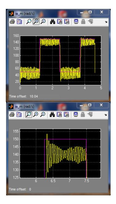
c) We then set the amplitude of the square wave to 0 to make the reference signal 100rad/s. We then ran the model and gently touched the load wheel to give the system a disturbance. Our screen shot is shown below.
