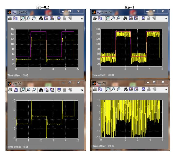
b) We then adjusted the K value until we found the system to be marginally stable. From this, we determined  $K_{pc}$  and  $T_{pc}$ . Our results and screen shots are shown below.
